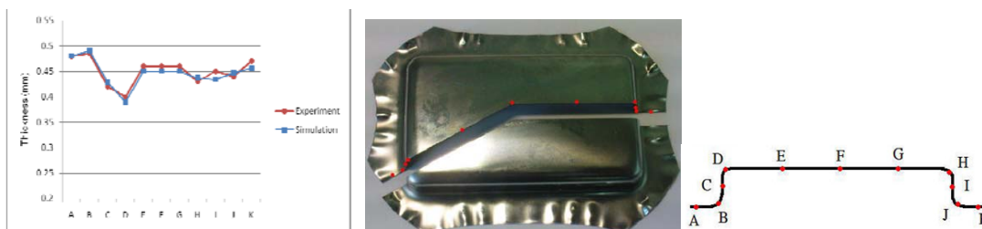
Figure 3 The verification of FE model with thickness distribution
