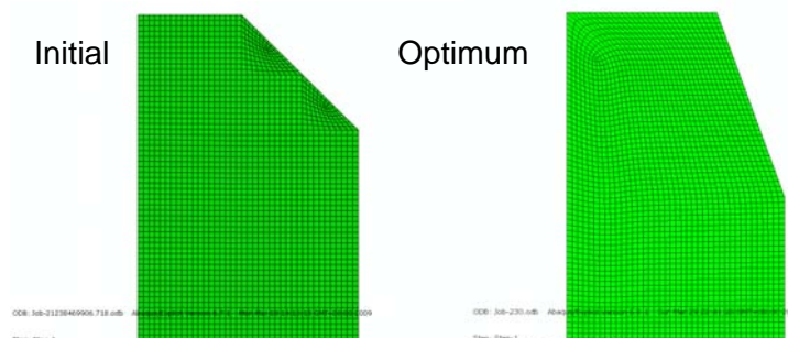
Figure 8 The comparison of initial and optimum blank shape
